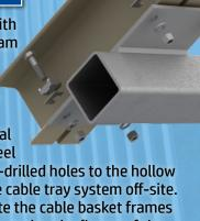
plates with four pre-drilled holes to the hollow section frame of the cable tray system off-site. Once delivered to site the cable basket frames would then be connected to the flange of the bridge steel channels using Type A girder clamps in a four-bolt configuration.
